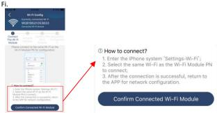
Enter the "Settings → Wi-Fi" and select connected Wi-Fi name. The connected Wi-Fi name is the same to your Wi-Fi PN number and enter default password "12345678".
